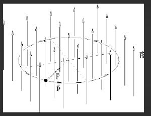
Motion of an electron (negative charge) in a uniform magnetic field.
